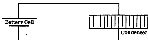
FIG. 204. The conventional diagram of a condenser connected to a battery cell.
